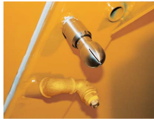
Rotating flushing nozzle(s) cleans the underside of the mixer lids.
