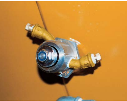
Horizontal flushing nozzle for cleaning the upper part of the gearbox and the mixing arms.
