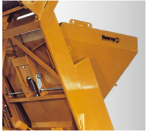
Automatic fall safety device for hoist bucket coming into effect immediately in case of a sudden slack wire.
