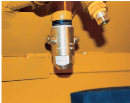
Vertical flushing nozzle for cleaning the side scraper and the lower part of the mixing arms.
