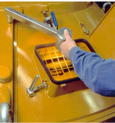
Lamp for inspecting the mixing cycle.
