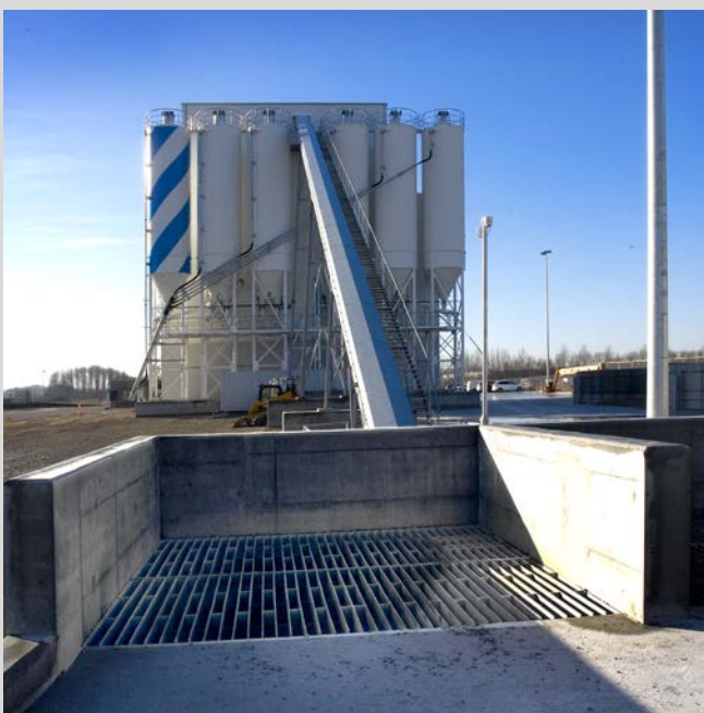
Hopper for tip loading with grating.
