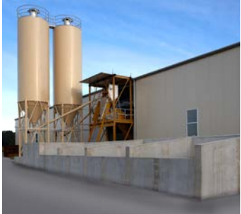
Precast plant with Haarup mixing plant and ground bins.
