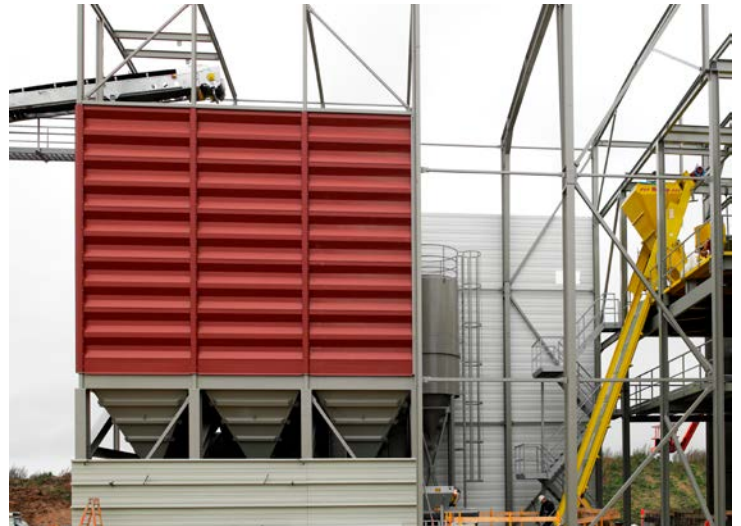
High silo system with filling system.
