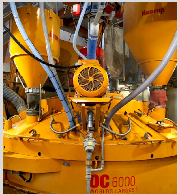
Water pump for intermediate cleaning of the mixer.
