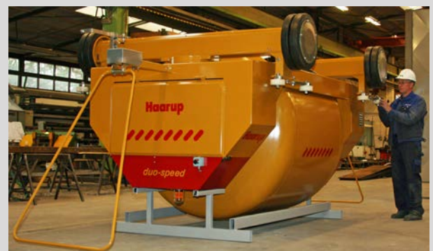
3500 litre duo-speed concrete travelling bucket is being tested before delivery.
