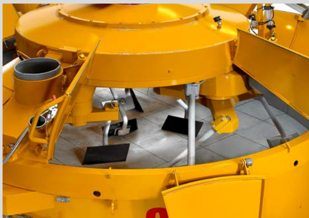
Side scraper, mixing arms, and mixing shovels in a 6000 litre mixer.
