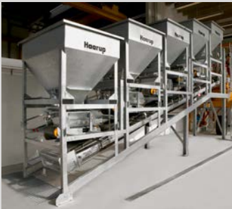
Small batching and mixing plant for Teknologisk Institut.
