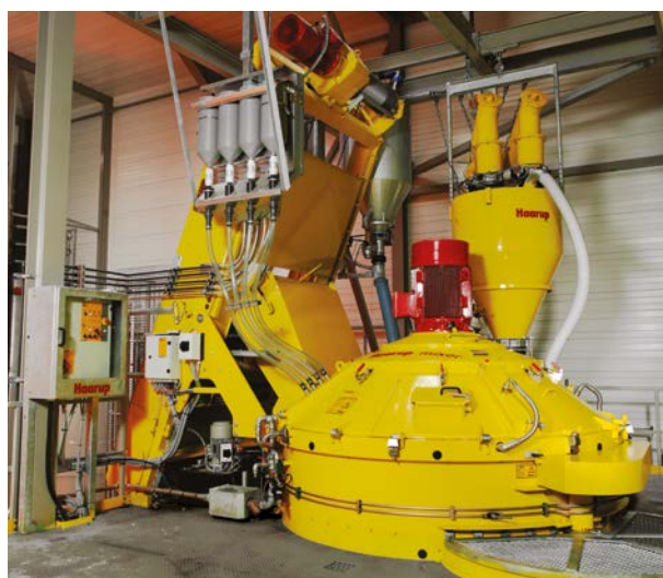
4-chamber admixture weigh hopper above a 2250 litre mixer.
