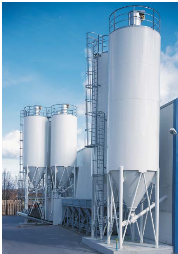
Cement silos with galvanized ladder, railing, and filter with pneumatic cleaning.
