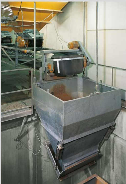
Combined weighing system with lattice weigh belt and weigh hopper.
