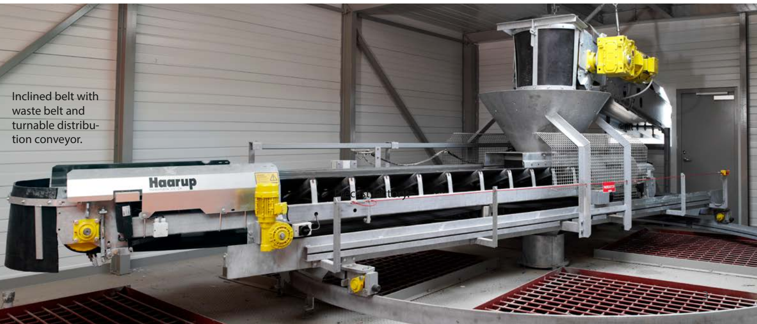
Modernisation of plant with new Haarup 3000 litre mixer.
