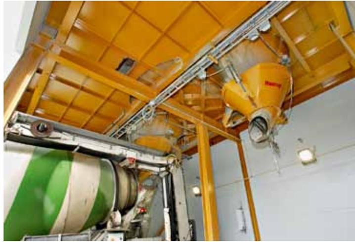
DK Beton decided in favor of installing a Haarup 6,000 liter mixer with two discharge units
