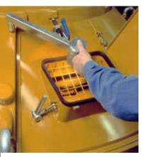
Lamp for inspecting the mixing cycle.
