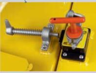
Mixer lids are fitted with relevant safety switch systems. When incorporated in the control system they will prevent the mixer running when the lids are opened.
