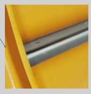
The plate covering of the mixing pan is designed with labyrinth seals ensuring optimum density and at the same time fast cleaning.
